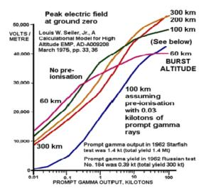
Typical HEMP curve, explaining how the peak EMP on the ground varies with weapon yield and burst altitude. (Photo above)
